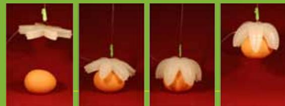
By using flexible, soft robotic tools, we have developed a general methodology, based on embedded pneumatic networks, enabling actuation of large soft elastomers, to create a universal gripper, shown here lifting an orange.
