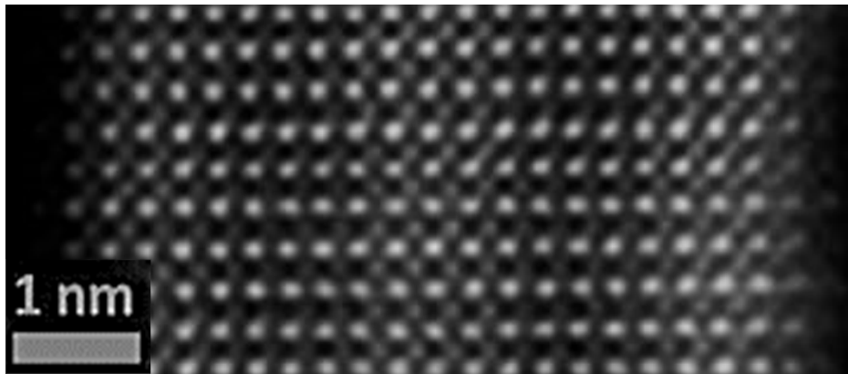
Epitaxial stack of coupled quantum wells
