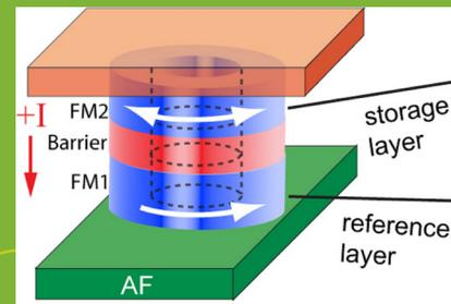
We have fabricated nanoring magnetic tunnel junctions with properties unattainable in disc-shaped MTJs.
