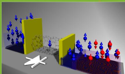
We have created a new type of spin diode with electrically controlled functionality using carbon nanotubes.
