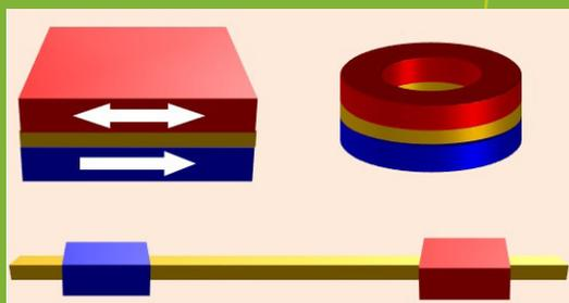
The JHU-MRSEC employs state-of-the-art techniques to fabricate and characterize inorganic and organic magnetoelectronic materials and devices such as perpendicular MTJs, nanorings, and lateral structures.
